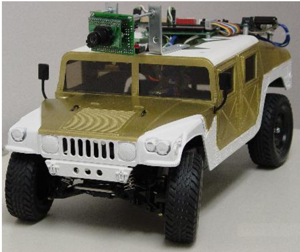
Figure 8: Student robot project controlled by an SoPC board with a camera and PWM servos
