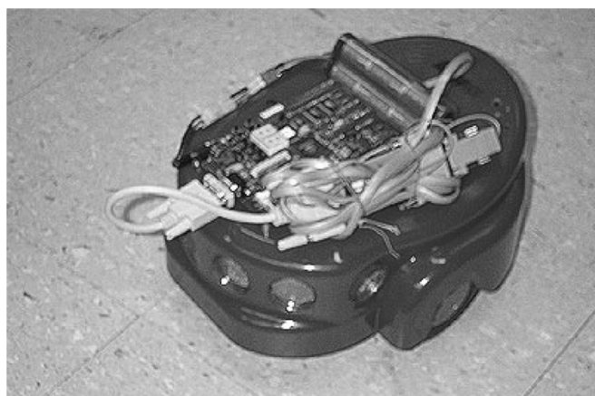
Fig. 6. Student project using the small Amigobot commercial robot controlled by the Altera Nios SOPC board.
