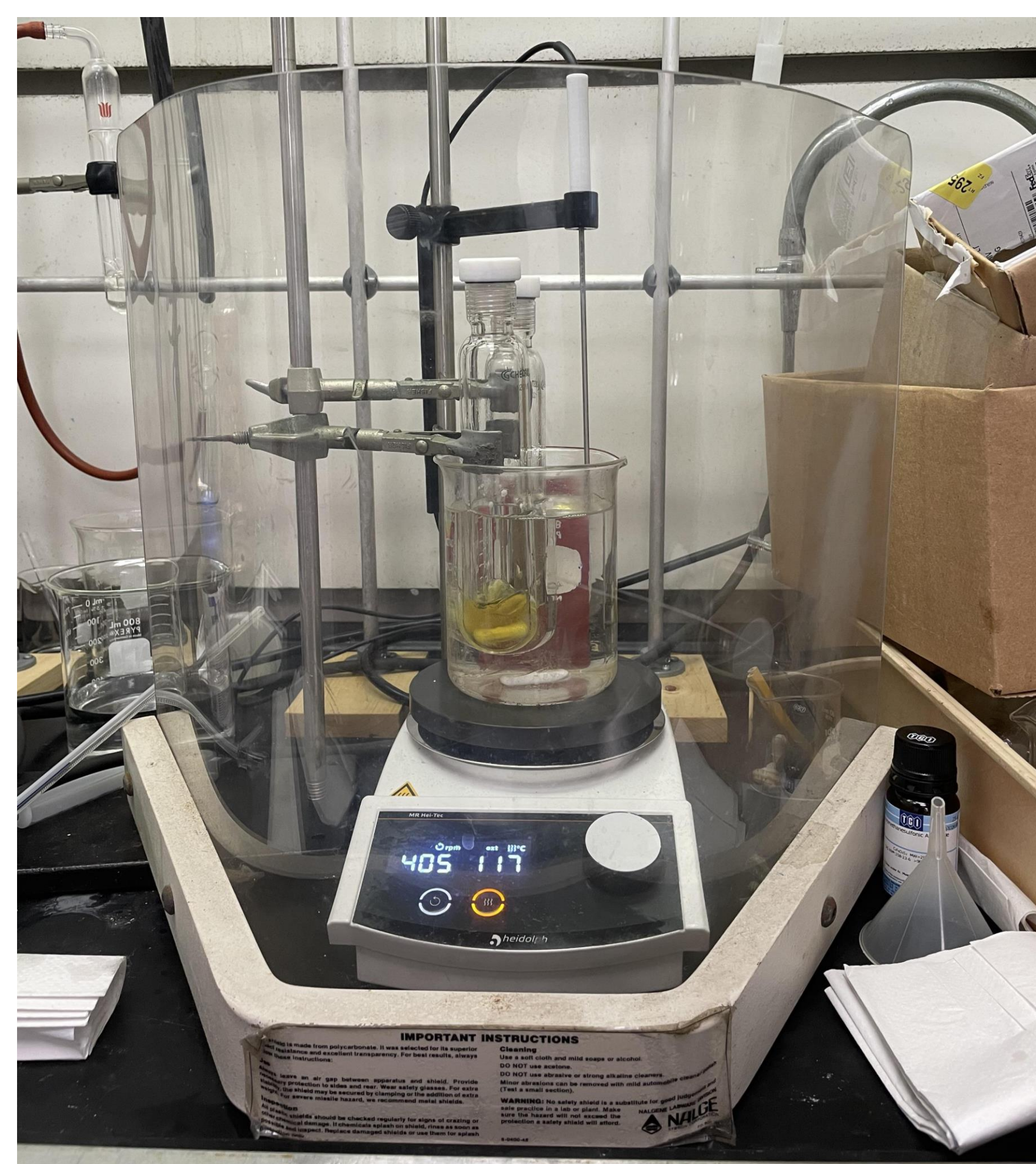
Figure 3. Reaction setup with the pressure tubes in an oil bath at 120°C behind a blast shield due to the reaction's pressure.
