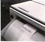
capital and lower case alphabets and other characters totalling 96 to each font. Each of these fonts is available in 12 sizes from keyboard control. The VIP justifies lines automatically and hyphenates with a fairly high degree of accuracy. A punched paper tape links the keyboards and typesetter.
