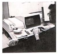
On the eve of our nation's 200th birthday, a fully computerized photocomposition system, including the Mergenthaler Variable Input Phototypesetter, known to the graphic arts world as the VIP, an Automix counting keyboard, as well as an editor and a Kodak processor, was installed. The VIP handles 18 typefaces at one time, including
