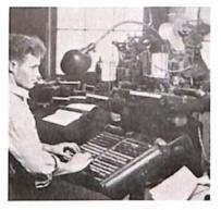
Somewhere around 1922-23 The Southern Publishing Association donated a Monotype typesetting system, consisting of the keyboard and caster. The system was a mechanical and typographical marvel. Each letter was a separate piece of type which made the type very hard to work with. The keyboard punched a paper controller tape which controlled the caster. Three pairs of capital and lower case alphabets in one size were available from one set up.
