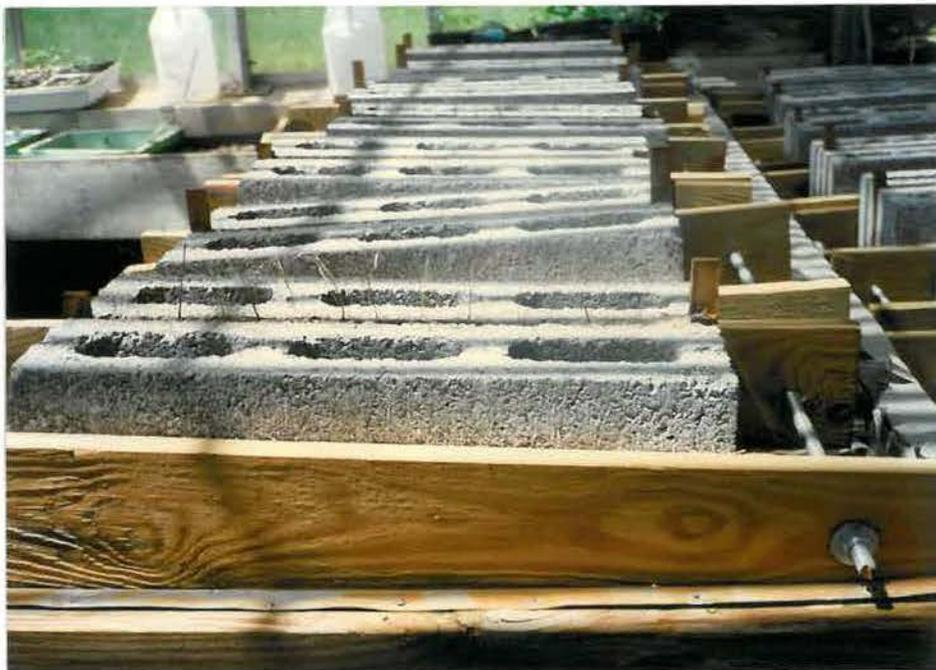
Figure 4. Simulation of natural environment using blocks in greenhouse.
