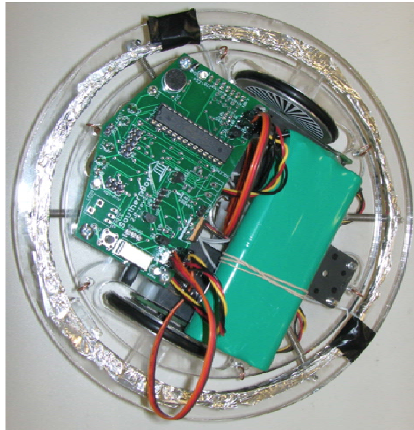
Figure 2. SouthernBot 2.0 is designed to be a flexible, very low-cost robot platform. It includes two continuous-rotation servo motors with custom rotation sensors as well as an omni-directional bump sensor, microphone, light sensor (phototransistor), and line-following sensor array.
